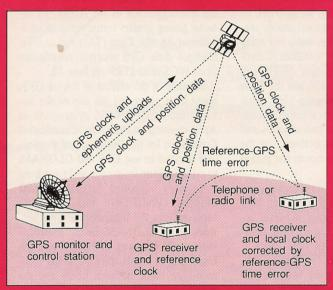
Figure 5: GPS common-mode common-view time transfer
