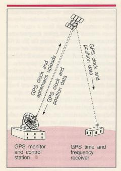
**Figure 1.** GPS time and frequency transfer
