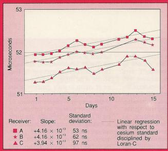
Figure 4: GPS 1PPS phase control
